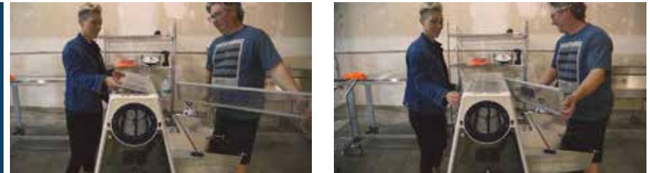
Close the lid and replace the clear top panel, brush and hex screens.
