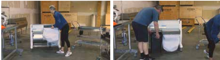
Reinstall the fan housing exhaust filter, the trim tote and the side panels.
