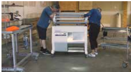
Reinstall the lid and connect the plug between the lid and the body
